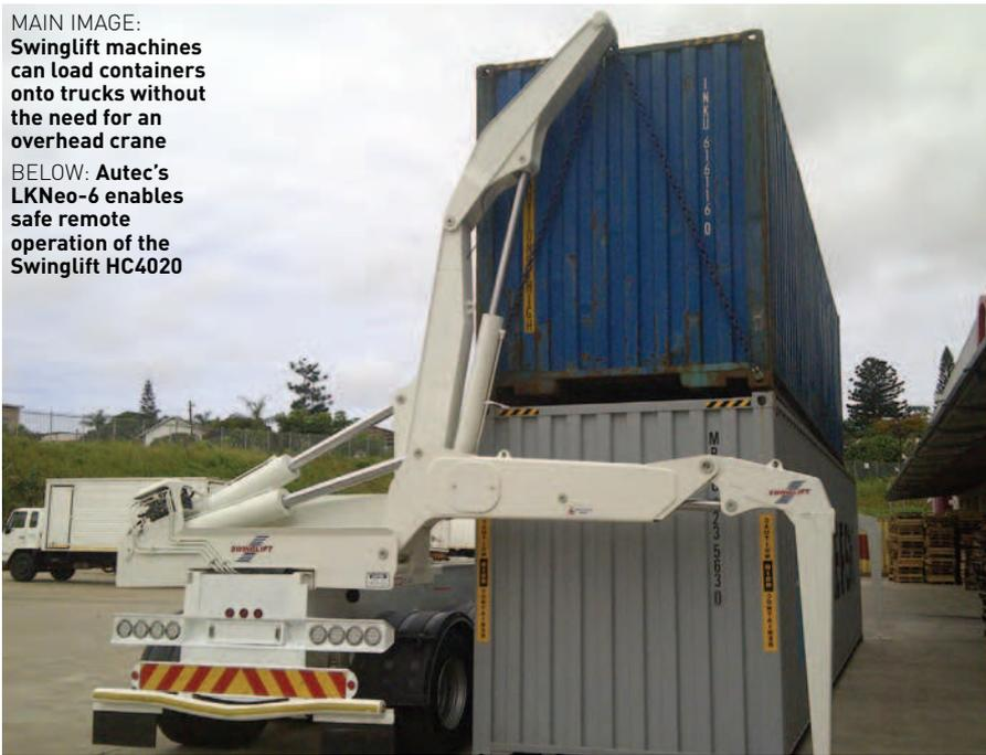
individually to get the correct deployment, especially on sloping ground. The operator can choose which stabilizers are operated using the 'Front-Both-Rear' toggle switch. The machine's control system calculates the position of the stabilizer foot using inclinometers, and can determine when the stabilizer is correctly deployed – either on the ground, or 'kneeling' on another truck for vehicle-to-vehicle loading.
